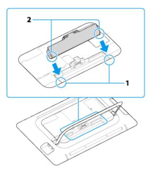
**7.** Turn the battery pack in the direction of the arrow and push the battery pack down into the compartment until it clicks into place.
